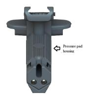
indexed intentionally. As such, the pressure pad keeper prevents accidental flash that would give away a soldier's location while in combat. The pressure pad keeper also prevents accidental activation while in storage, reducing costs in batteries and increasing reliability.
